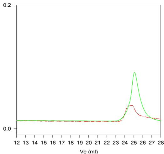
Size exclusion chromatography of poly(ethylene oxide-b-t-butyl methacrylate)
