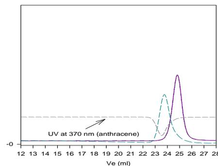
Polystyrene, M<sub>n</sub>=11500, M<sub>w</sub>=12100 PI=1.05
