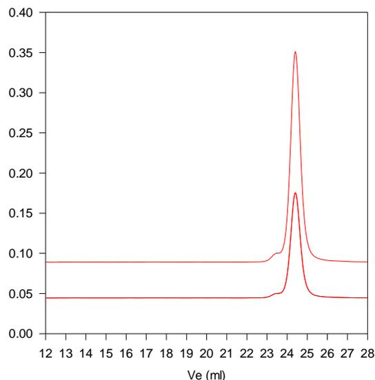
Size exclusion chromatography of polystyrene terminated with dimethyl chlorosilane before and after termination with dimethyl dichlorosilane:
