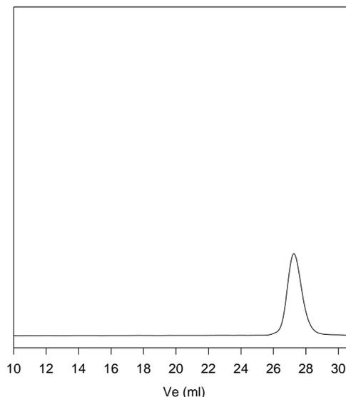
Size exclusion chromatography of dicarboxy terminated polybutadiene before termination with  $\text{CO}_2$ :
