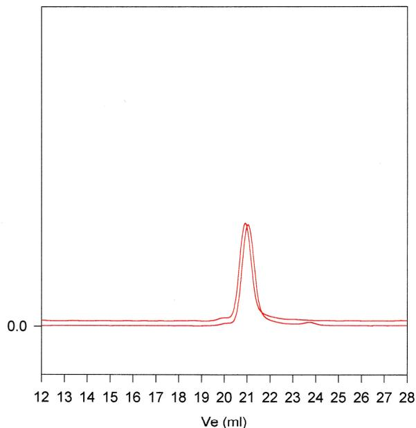
Size exclusion chromatography of polystyrene terminated with dimethyl chlorosilane before and after termination with dimethyl dichlorosilane:
