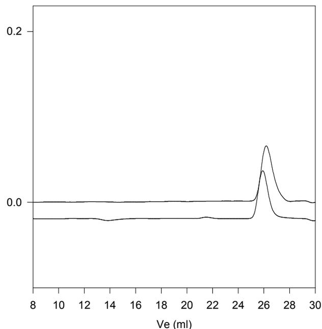
Size exclusion chromatography of poly(ethylene oxide-b-butylene oxide)
