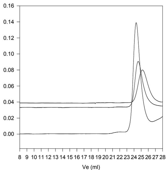
Size exclusion chromatography of poly(t.butyl methacrylate-b-ethylene oxide)
