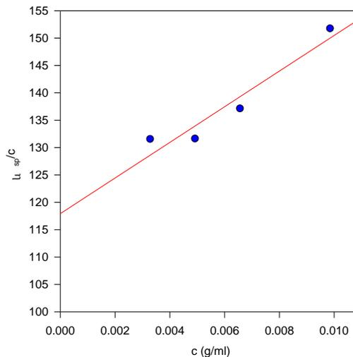
Intrinsic Viscosity measurement of Poly(N-isopropyl acrylamide) in Methanol at 25°C
