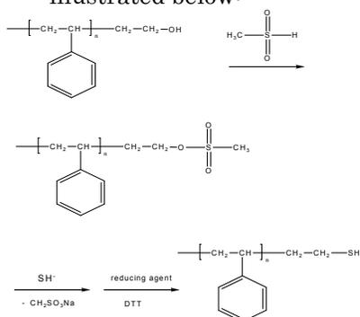
2. From direct termination of anionic living polymerization of styrene by ethylene sulfide or propylene sulfide. Polymerization of styrene by Sec.BuLi in THF at -78 °C and termination by purified ethylene sulfide or propylene sulfide.
