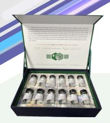
Our POLY (STYRENE) standards kit includes 12 samples with molecular weight ranging from 800 Da to 6,000,000 Da and narrow polydispersity. All our Certified Reference Materials conform to international quality standards and are good for calibration and evaluation of analytical instruments, as well as for fundamental research.
